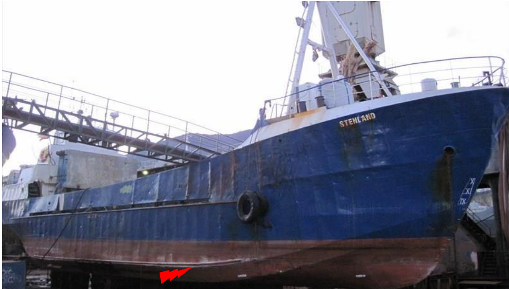
Figure 6. Stella in dry dock, located in the Adriatic Sea. The starboard bottom section that was reported to have been damaged and holed (photo source marine traffic taken on 08-03-2012).
